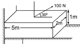
Sol. Longitudinal or normal stress  $\Rightarrow \sigma_l = \frac{100 \sin 30^\circ}{5 \times 2} = 5 \text{ N/m}^2$
