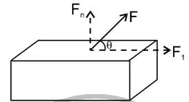
$$\therefore \text{Normal (tensile) stress} = \frac{F_n}{A} = \frac{F \sin \theta}{A}$$
