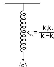
Get Solution of These Packages & Learn by Video Tutorials on [www.MathsBySuhag.com](http://www.MathsBySuhag.com) for the system of rods shown in figure (a), the replaced spring system is shown in figure (b) two spring in series]. Figure (c) represents equivalent spring system. Figure (d) represents another combination of rods and their replaced spring system.
