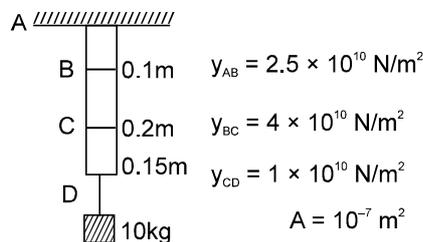
**Sol.**  $\Delta L_B = \Delta L_{AB} = \frac{FL}{AY} = \frac{MgL}{AY} = \frac{10 \times 10 \times 0.1}{10^{-7} \times 2.5 \times 10^{10}} = 4 \times 10^{-3} \text{ m} = 4 \text{ mm}$
